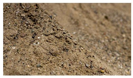
2NS sand, or "sharp sand" as it can be called, is a natural product that has been washed, leaving it free from any foreign debris such as clays and dirts. The sand is 3mm in size and should pass through a #6 sieve, but not a #8 sieve. The sand is not weathered, giving it the "sharper" corners to lock and bind better.
